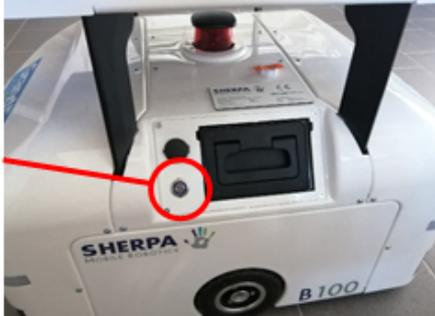
A close-up photograph of the Sherpa B100 control panel. A red circle highlights the power button, which is a small circular button with a power symbol. A red line points from the circle to the button. The panel also features a larger screen and other controls. |
