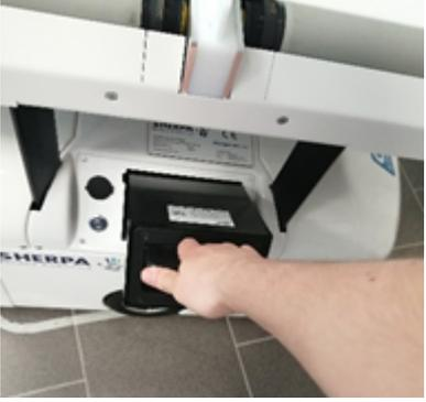
A close-up photograph of a hand pulling the black battery out of the bottom of the white Sherpa device.                                                                                                                                                                            |
